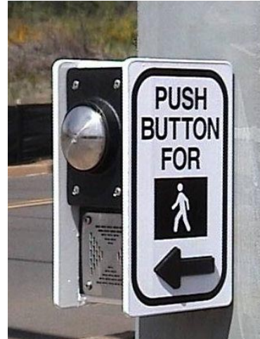
FIG. 15-2. CAMPBELL APS H-FRAME VERSION IS USED IN SOME NORTHWESTERN CITIES SO THAT THE PUSHBUTTON CAN BE MOUNTED ON THE SIDE OF THE POLE AWAY FROM THE STREET. HOWEVER, THE H-FRAME BLOCKS THE SOUND FROM THE SIDES OF THE APS, MAKING IT LESS USABLE FOR HOMING IN ON THE LOCATOR TONE.
