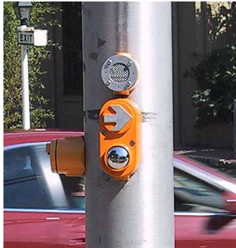
FIG. 12-7. DIRECTION OF THE CAST-IN-PLACE ARROW ON THIS DEVICE MUST BE SPECIFIED WHEN ORDERING.
