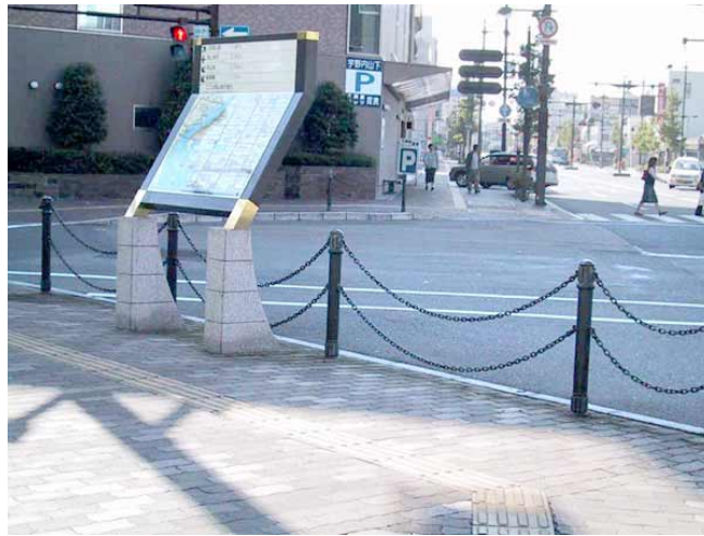
FIG. 4-2. AT THIS INTERSECTION A CHAIN FENCE IS USED WHERE CROSSING IS PROHIBITED
