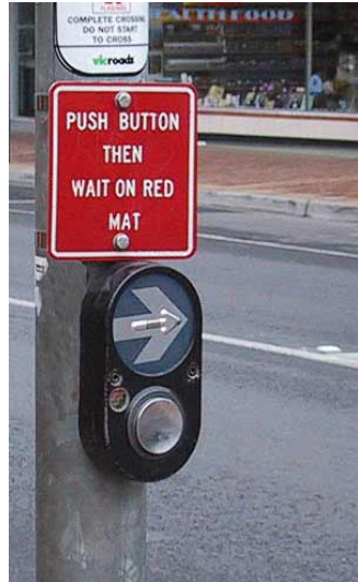
FIG. 7-10. (LEFT) DETAIL OF APS AT MIDBLOCK CROSSING IN AUSTRALIA. SIGN READS "PUSH BUTTON THEN WAIT ON RED MAT."
