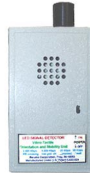
FIG. 15-13. RELUME PERSONAL RECEIVER PLAYS A RECORDED SPEECH MESSAGE WHEN TRIGGERED BY THE RELUME PEDHEAD.
