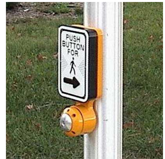
FIGS. 5-5 AND 5-6. TWO EXAMPLES OF PUSHBUTTON-INTEGRATED APS WITH AUDIBLE AND VIBROTACTILE OUTPUT. BOTH HAVE LOCATOR TONES AS WELL AS WALK INDICATIONS.
