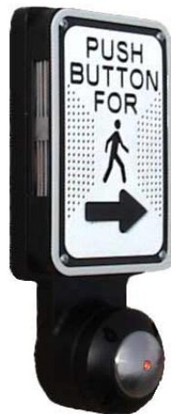
FIG. 7-1. THIS APS HAS A LARGE, HIGH CONTRAST, TACTILE ARROW ABOVE THE PUSHBUTTON. THE ARROW VIBRATES RAPIDLY DURING THE WALK INTERVAL.
