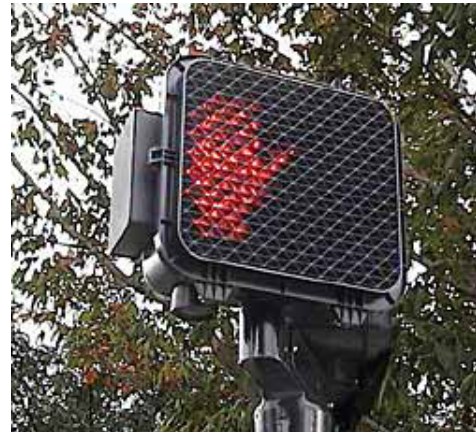
FIG. 12-3. EXTERNAL MOUNT FOR CONTROLLER BOARD IS VISIBLE ON THE LEFT SIDE OF THE PEDESTRIAN SIGNAL HEAD.
