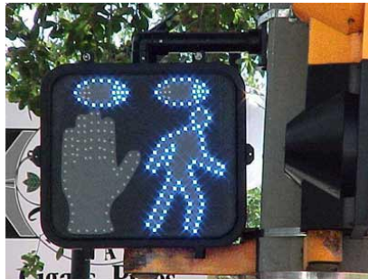
FIG. 5-9. THE PULSING OF THE LEDs IN THE PEDHEAD ACTIVATES A SPEECH MESSAGE IN A HANDHELD RECEIVER.
