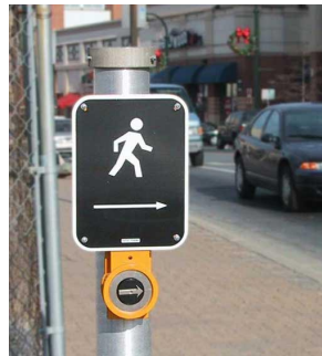
FIGS. 5-5 AND 5-6. TWO EXAMPLES OF PUSHBUTTON-INTEGRATED APS WITH AUDIBLE AND VIBROTACTILE OUTPUT. BOTH HAVE LOCATOR TONES AS WELL AS WALK INDICATIONS.
