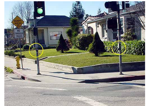
FIG. 11-2. WELL LOCATED PEDESTRIAN SIGNAL POLES PROVIDE APS AUDIBLE INDICATIONS FROM THE OPTIMAL LOCATION, CLOSE TO THE PEDESTRIAN WAITING AREA.
