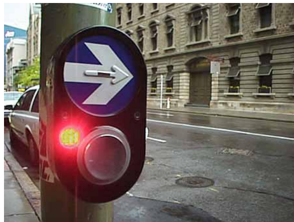
FIG. 7-3. THE VIBRATING TACTILE ARROW ABOVE THE PUSHBUTTON ON THIS APS IS SUPERIMPOSED ON A LARGER VISUAL ARROW.
