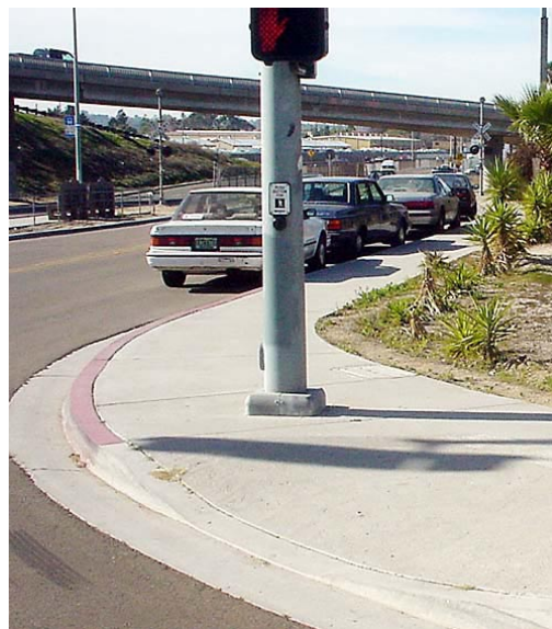
FIG. 10-3. THE FACE OF THE DEVICE SHOULD BE ORIENTED TOWARD THE INTERSECTION
