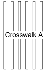
FIG. 12-34. POSSIBLY ACCEPT-ABLE PLACEMENT FOR PEDHEAD-MOUNTED APS ON THE OUTSIDE OF THE PEDHEADS. PROVIDE AS MUCH SEPARATION AS POSSIBLE.
