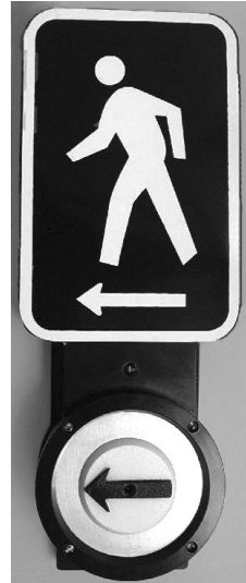
FIG. 15-9. THE NAVIGATOR APS HAS A LARGE PUSH- BUTTON THAT INCLUDES A VIBROTACTILE ARROW. A SMALL DEPRESSION IN THE ARROW ENABLES PUSHBUTTON OPERATION WITH A HEAD STICK.
