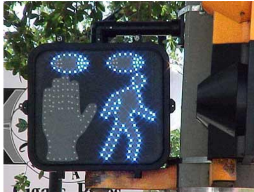
FIG. 15-12. THE PULSING OF THE LEDs IN THE RELUME PEDHEAD ACTIVATES A SPEECH MESSAGE IN A HANDHELD RECEIVER.
