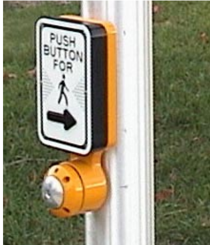
FIG. 15-1. THE CAMPBELL IQ APS HAS A LARGE, CONVEX PUSHBUTTON WITH A SMALL INDENTATION IN THE CENTER SO THAT IT CAN BE ACTUATED WITH A HEAD-STICK USED BY A PERSON HAVING NO LIMB DEXTERITY. THE LARGE ARROW ABOVE THE PUSHBUTTON IS VIBROTACTILE.
