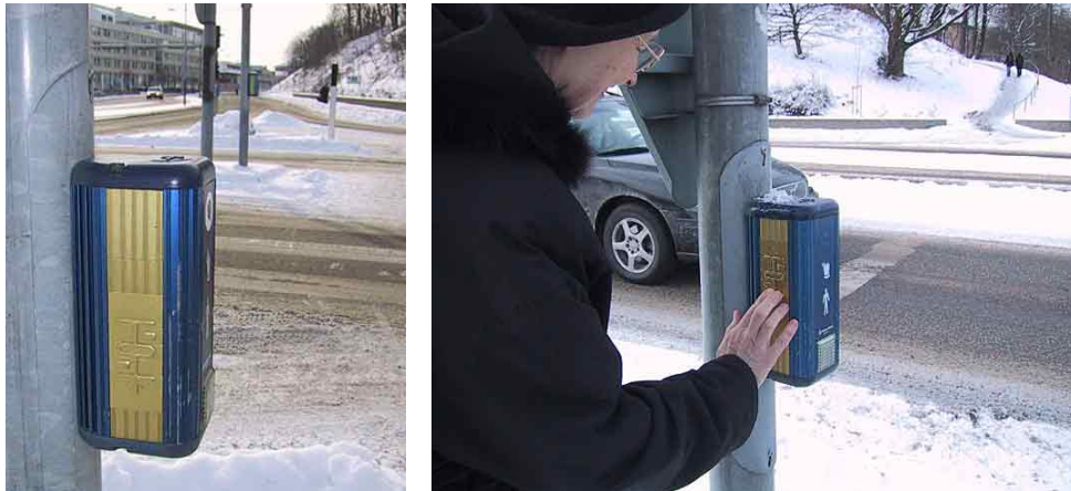
FIG. 4-12 AND 4-13. THE APS DISPLAYS A TACTILE MAP ON ONE SIDE.
