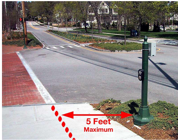
FIG. 10-4. THE APS SHOULD BE WITHIN 5 FEET OF THE CROSSWALK LINE EXTENDED.
