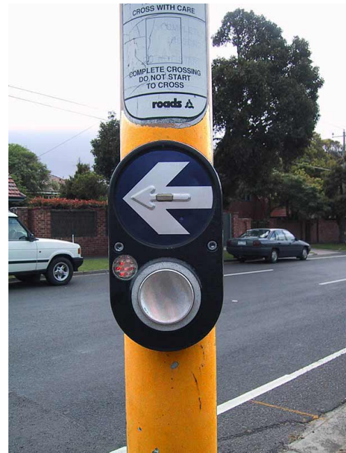
FIG. 4-7. THIS APS HAS A TACTILE ARROW WITHIN A LARGER VISIBLE ARROW. OTHER FEATURES INCLUDE A LOCATOR TONE AND AUDIBLE AND VIBROTACTILE WALK INDICATION
