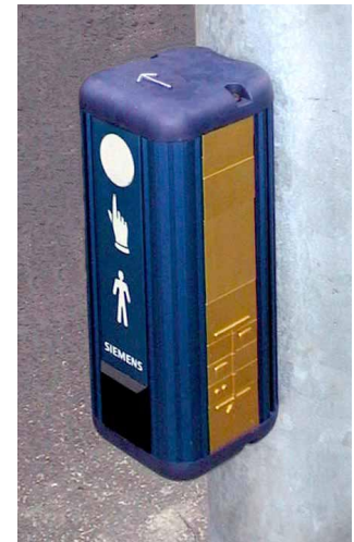
FIG. 7-1. THIS APS HAS A LARGE, HIGH CONTRAST, TACTILE ARROW ABOVE THE PUSHBUTTON. THE ARROW VIBRATES RAPIDLY DURING THE WALK INTERVAL.
