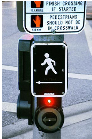
FIG. 7-5. A RED ACTUATION INDICATOR LIGHT IS ABOVE THE PUSHBUTTON.
