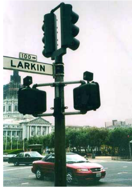
FIG. 5-10. PEDHEAD-MOUNTED APS UNITS TRANSMIT SPEECH MESSAGES TO A HANDHELD RECEIVER.
