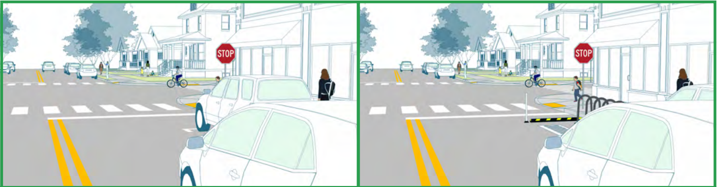
Daylighting improves visibility of pedestrians by removing parked cars next to crosswalks and opening the field of vision for all road users at intersections. Drawing on left shows view without daylighting. Drawing on right shows view with daylighting.
