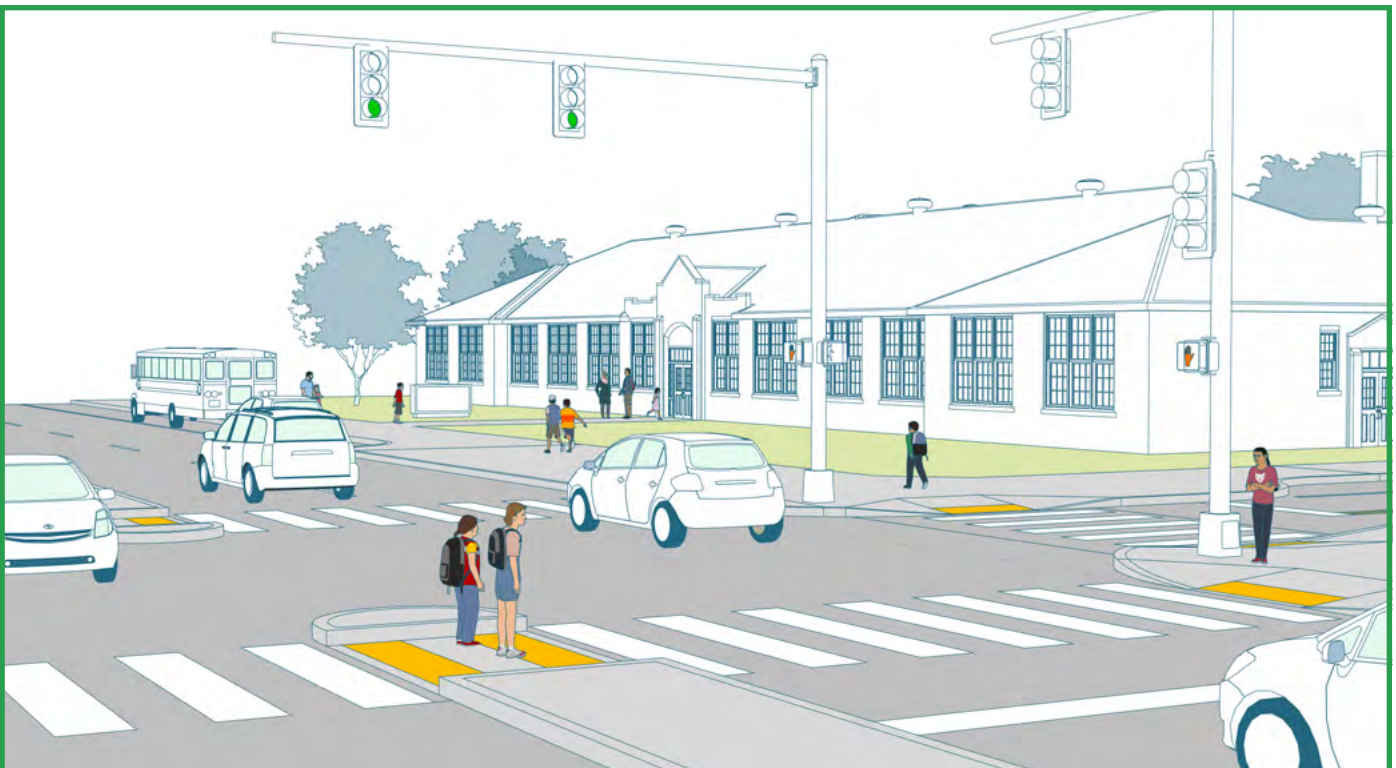
Crossing islands simplify street crossings by allowing pedestrians to assess and cross one direction of traffic at a time while also reducing the amount of time pedestrians are in the path of traffic.
