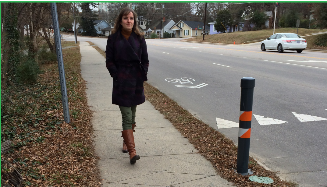
Figure 2. Inductive loop bicycle counter on road and sidewalk and passive infrared counter on sidewalk counts pedestrians and bicyclists on sidewalk plus bicyclists on the road in Chapel Hill, North Carolina.
