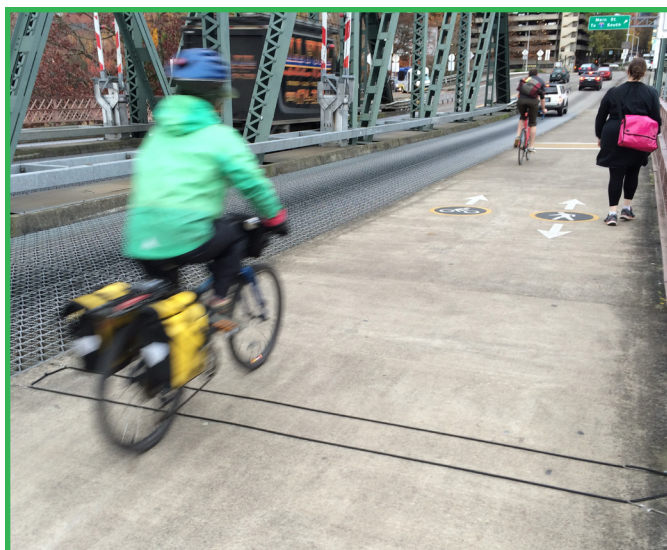
Figure 4. Pneumatic tube bicycle counter used as a permanent continuous counter on the Hawthorne Bridge in Portland, Oregon. (Source: Krista Nordback)
