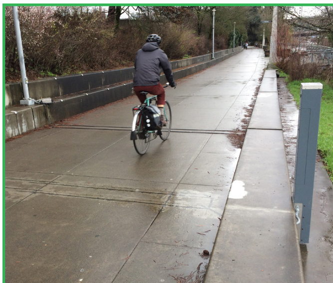
Figure 7. Bicycle counts from a permanent piezoelectric bicycle counter (combined with passive infrared pedestrian and bicycle counter) being validated using a pneumatic tube counter on a shared use path in Portland, Oregon. (Source: www.pedbikeimages.org/ Krista Nordback)
