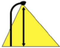
Luminaire mounting height
