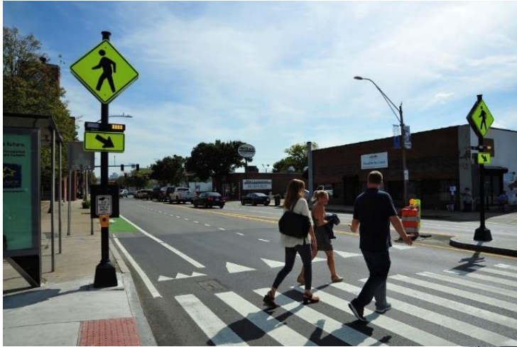
Rectangular Rapid Flashing Beacon (RRFB)
