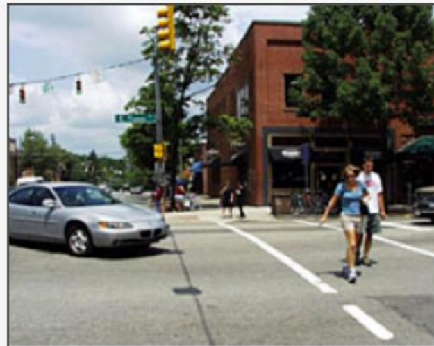
Pedestrians may conflict with left-turning vehicles when permissive signal phasing is used.
