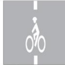
Bike detector pavement marking MUTCD Fig. 9C-7
