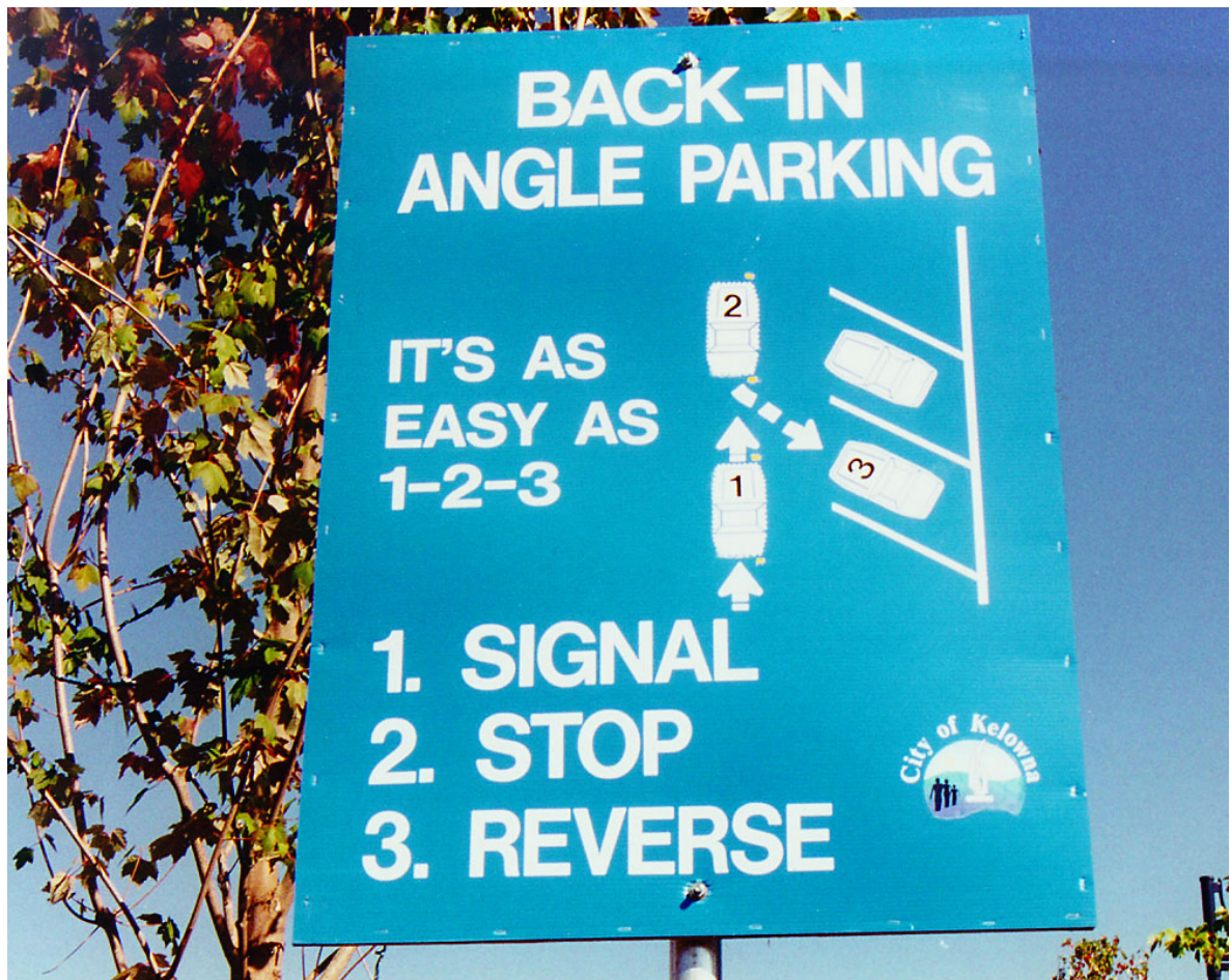
Figure 5 A traffic sign showing the three steps of back-in angle parking, in Kelowna, BC, Canada.
