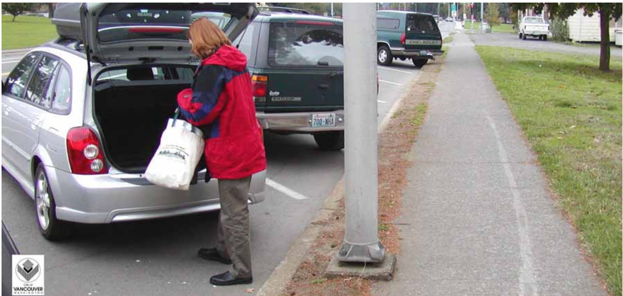
Figure 2 With back-in angle parking you can load your car on the curb, rather than in the street (Vancouver, WA).
