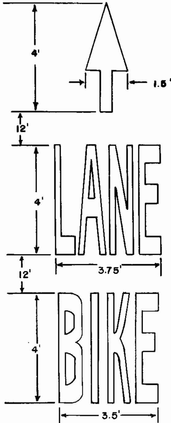
**Figure D-5 Class II Bikeway Lane Marking**
