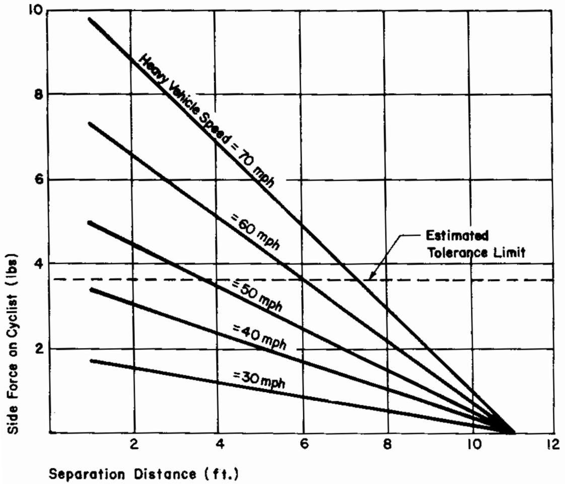
Figure B 1 Aerodynamic Forces on Cyclists
