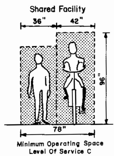
Figure C-9 Lateral And Vertical Bikeway Clearances
