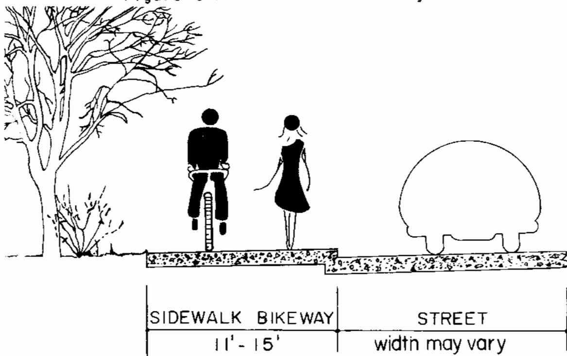
Figure C-2 Class I Sidewalk Bikeway
