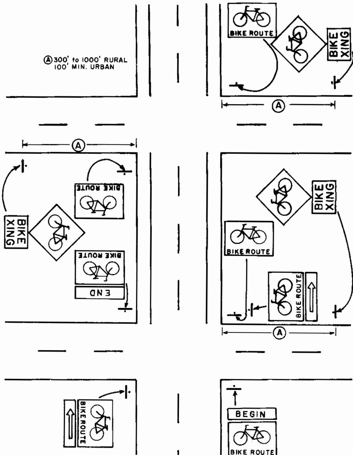
Figure D-3 Class II & III Bikeway Signing
