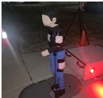
Figure 1. Photograph. An articulated child pedestrian dummy configured for thermal testing for the Enhancing VRUs project.
