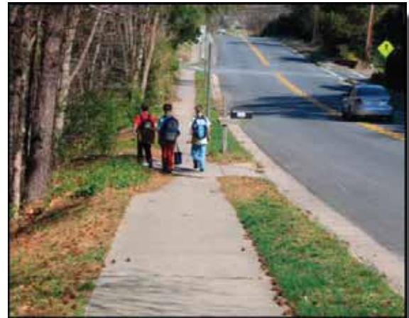
Although a narrower sidewalk might be adequate for many pedestrian uses, school children may require additional space since they often walk in groups. Insufficient sidewalk width can be a particular concern for younger children, who are easily distracted. In such situations, a wider sidewalk can greatly improve safety. This photo shows that a 5 foot wide sidewalk is barely sufficient for even a small group of school children, though the landscaped buffer strip provides additional separation from traffic.
