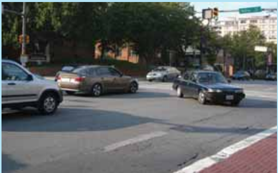
The two photos show a vehicle making a permissive left turn in front of oncoming traffic and nearly hitting pedestrians in a crosswalk during the WALK interval. The RSA team may suggest providing a protected left turn that does not conflict with the pedestrian WALK interval.
