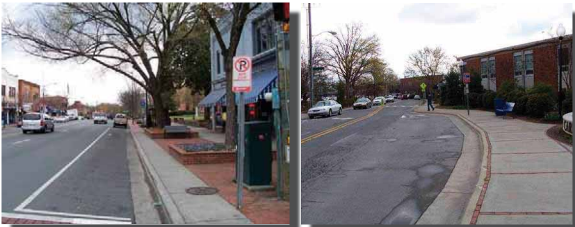
In the photo on the left, buses stop in a no-parking area, while in the photo on the right, buses stop in a bus bay. Both stops effectively separate transit riders from other modes of travel.
