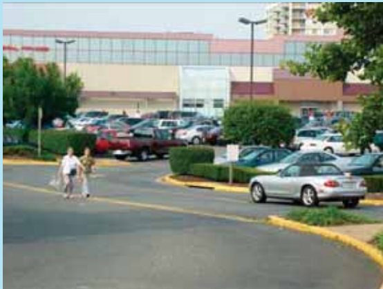
Pedestrians in the parking lot of a shopping mall are walking in the roadway where they may conflict with vehicles. The absence of sidewalks or clear pedestrian pathways exposes pedestrians to the risk of collision with drivers who are often distracted by the need to find a parking spot.
