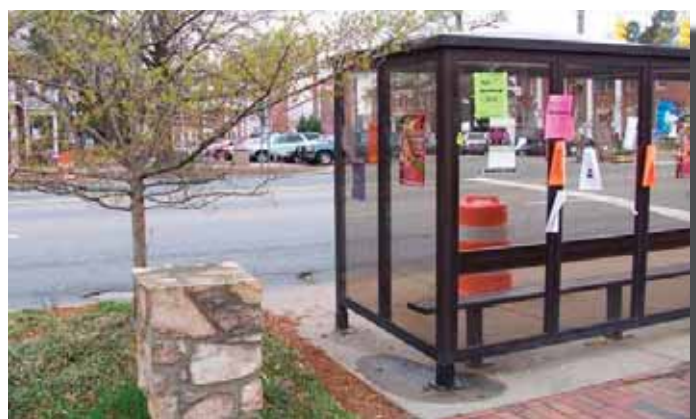
The photo on the left shows access to a bus stop (in the distance) obstructed by a telephone pole. Access to the bus shelter on the right is inhibited due to a missing connection between the sidewalk and the bus shelter landing.
