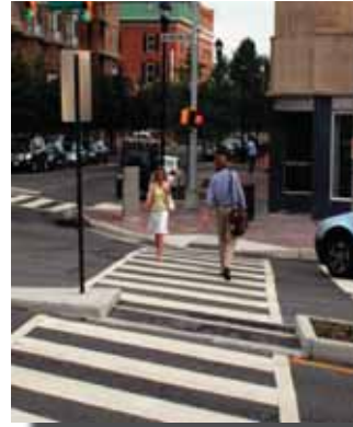
Curb ramps and cut throughs are oriented directly in line with the crosswalks, so that pedestrians do not need to walk outside the crosswalk markings when entering or leaving the crosswalk. The ramps correctly orient pedestrians with low vision along the crosswalk alignment when they are entering the crosswalk.
