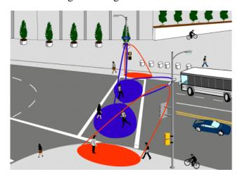
When used at the curbside area, they may either replace or augment the standard push button used to activate the pedestrian call feature. When used to detect pedestrians in the crosswalk, the function is to detect the presence of individuals requiring additional time to cross and, accordingly, extend the clearance interval and provide more time to cross.
