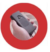
receivers. Talking Signs® is a product of this type. Messages may identify the location and direction of travel of the pedestrian, give the name of the street to be crossed, and provide real time information about WALK and DON'T WALK intervals. It is an infrared wireless communications system that is designed to work in both interior and exterior applications and makes confident independent travel possible for visually impaired
