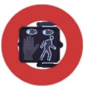
encourage pedestrians to look for turning vehicles traveling on an intersecting path by including a prompt as part of the pedestrian signal. The prompt is a pair of animated eyes that scan from side to side at the start of the WALK indication.
