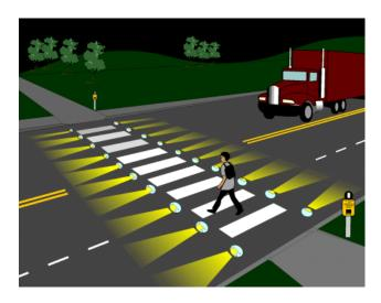
both sides of the crosswalk and oriented to face oncoming traffic. When the pedestrian activates the system, either by using a push-button or through detection from an automated device, the lights begin to flash at a constant rate, warning the motorist that a pedestrian is in the vicinity of the crosswalk ahead.
