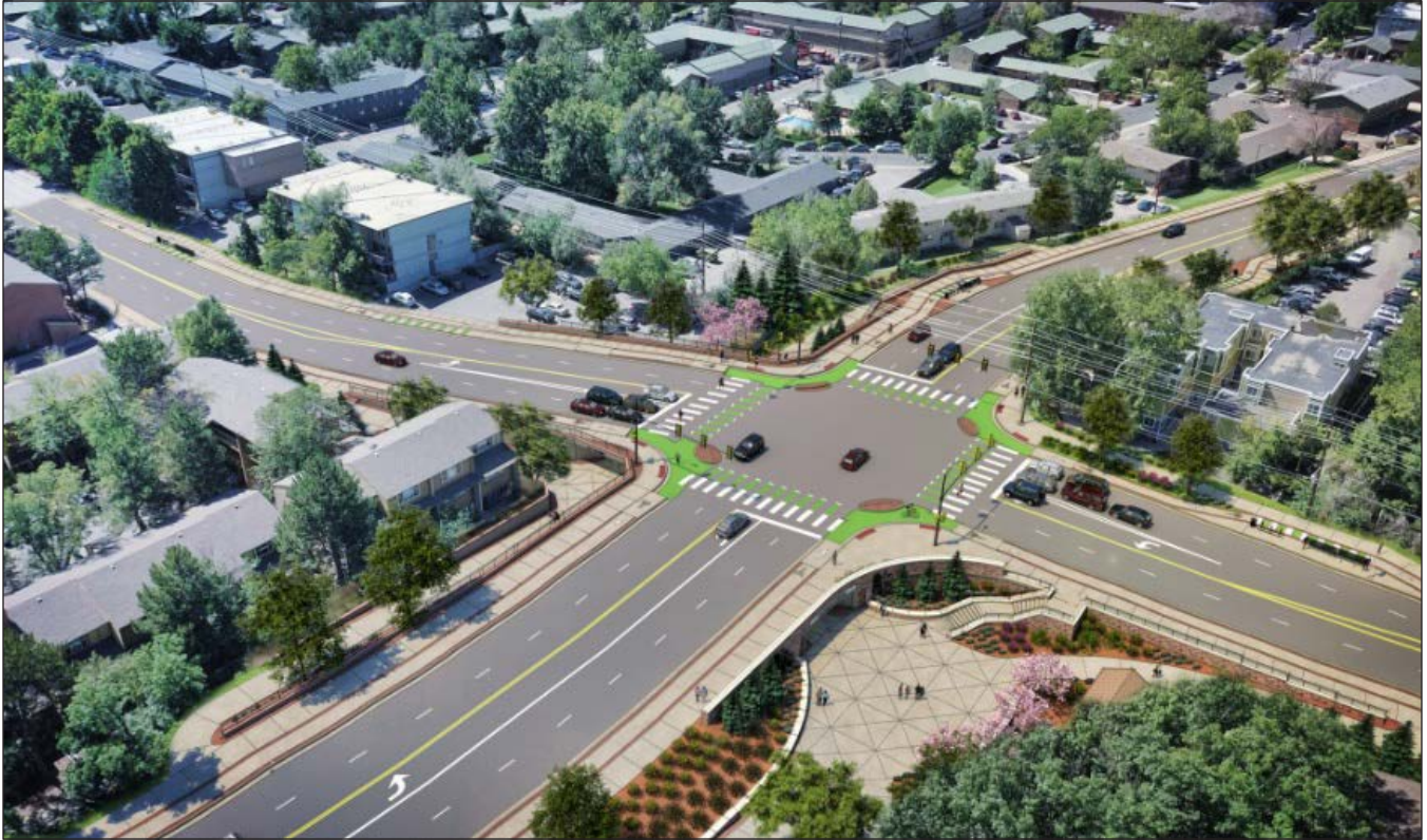
Figure 3. Image. Rendering of 30th Street and Colorado Avenue intersection improvements (protected intersection, underpasses) under construction.
