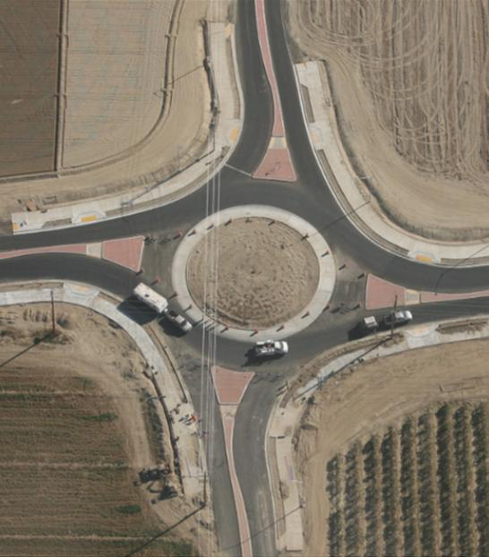
Figure 7. Single lane roundabout in a rural area. Source: Caltrans
