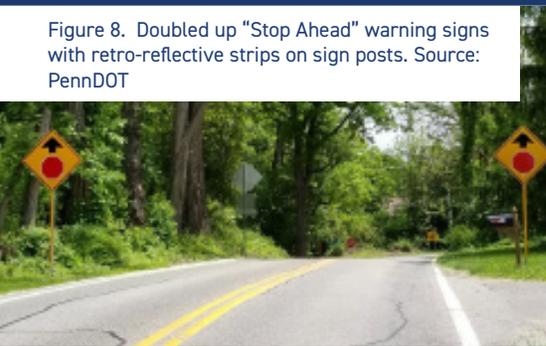
Figure 8. Doubled up "Stop Ahead" warning signs with retro-reflective strips on sign posts. Source: PennDOT
