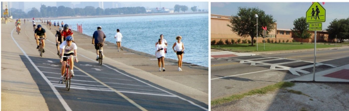
Examples of active transportation infrastructure, including a shared-use path and a raised crosswalk. Source: Left image source: pedbikeimages / Dan Burden; right image source: pedbikeimages / Dan Burden
