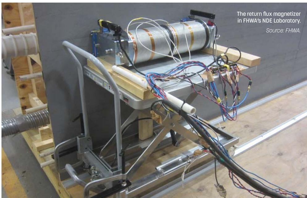
cover in actual post-tensioned structures plus an air gap between the yoke bottom and concrete surface.
