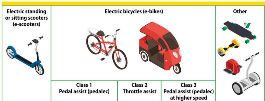
Examples of powered micromobility devices and their classifications according to PBIC.
