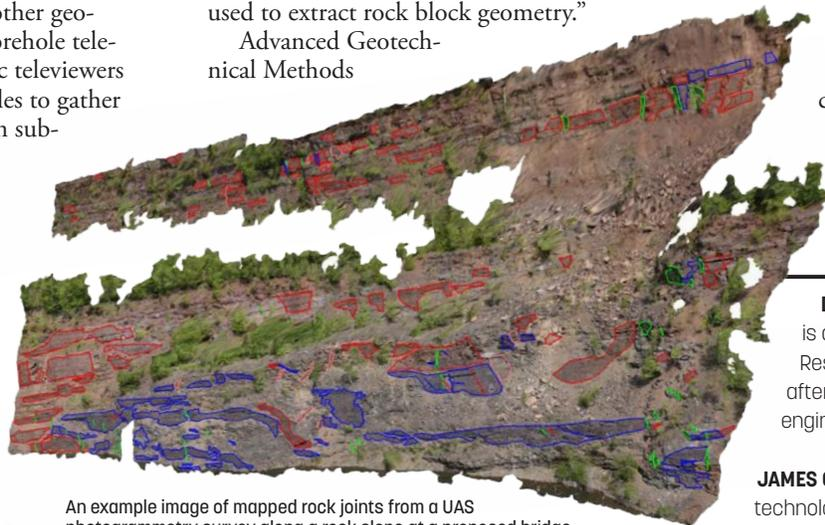
An example image of mapped rock joints from a UAS photogrammetry survey along a rock slope at a proposed bridge location on the U.S. 53 relocation project in Virginia, MN.
