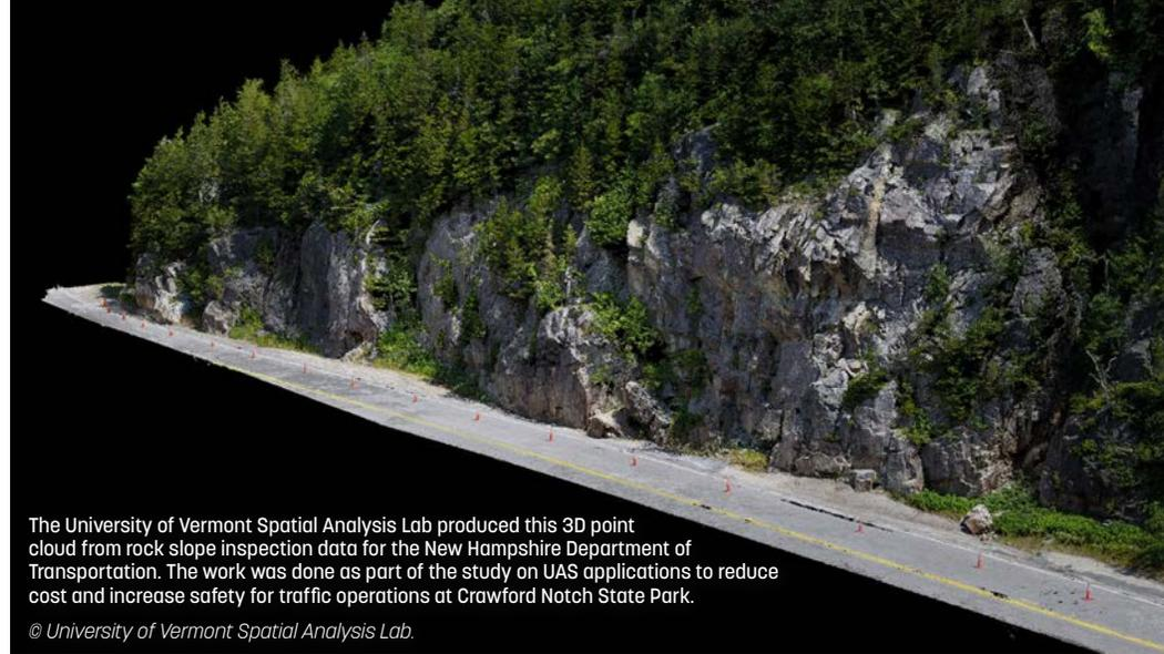
The University of Vermont Spatial Analysis Lab produced this 3D point cloud from rock slope inspection data for the New Hampshire Department of Transportation. The work was done as part of the study on UAS applications to reduce cost and increase safety for traffic operations at Crawford Notch State Park.
