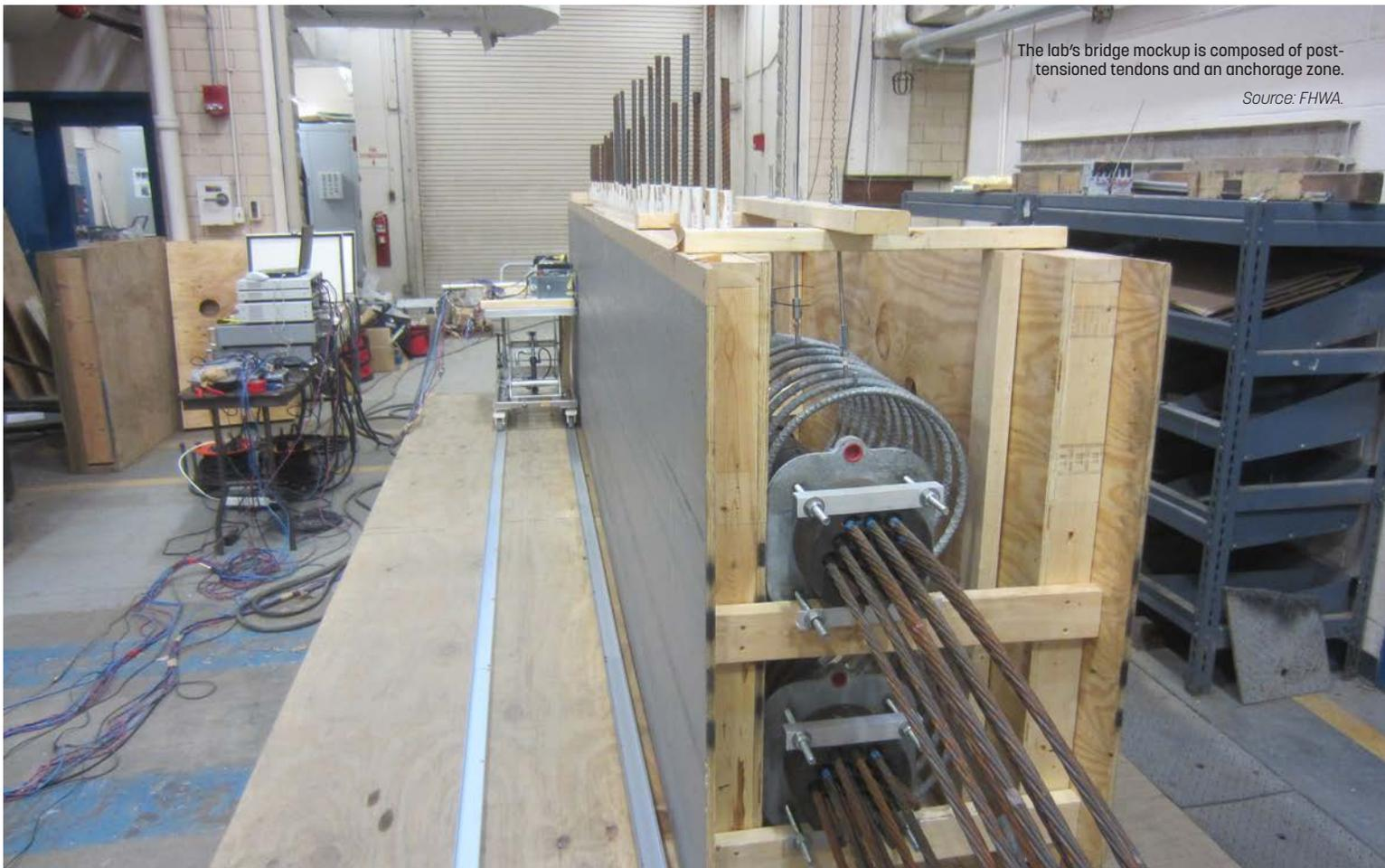
The lab’s bridge mockup is composed of post-tensioned tendons and an anchorage zone.
