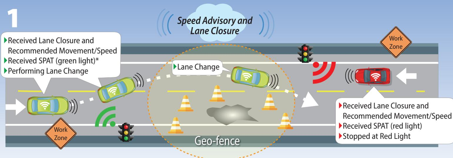
The first work zone management use case involves a one-lane, two-way traffic taper. Vehicles traveling on the side of the road blocked by the work zone must merge into the lane traveling in the opposite direction.
