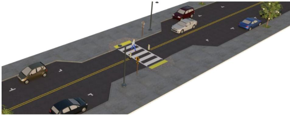
Figure 25. Graphic. Concept demonstrating curb extensions on both sides of crosswalk (VHB, 2018).\*
