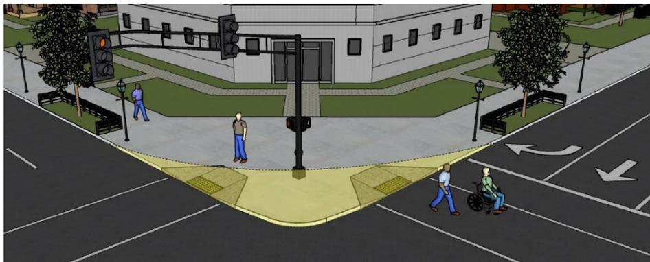
Figure 26. Graphic. Concept showing reduced corner radii (VHB, 2021).\*
