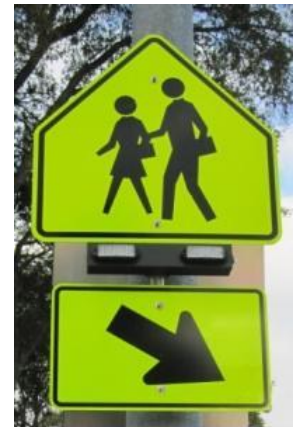
Figure 3. Example of the rectangular rapid flashing beacon being used with school sign. Source: Texas Transportation Institute.
