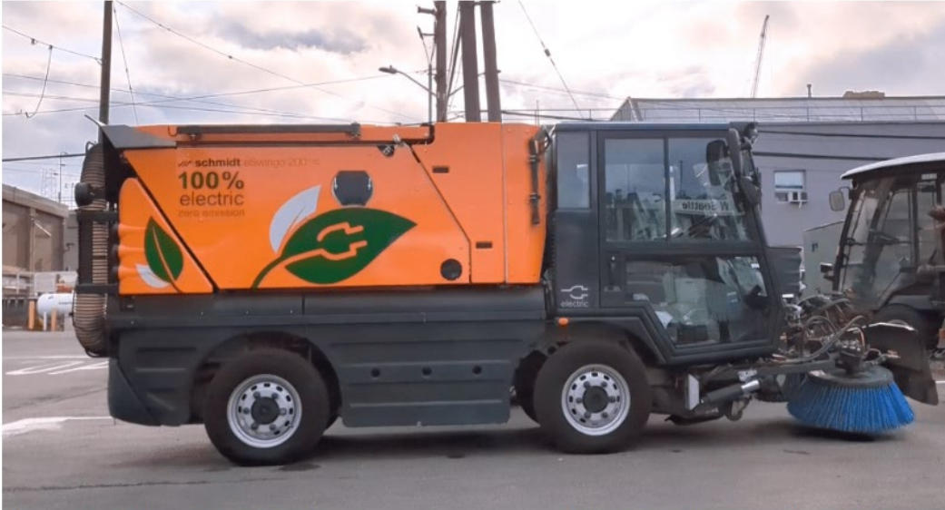
Pictured: eSwingo 200+ electric compact sweeper rented by SDOT. Photo Credit: SDOT.
