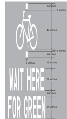
Figure 9E-16. Bicycle Detector Pavement Marking
